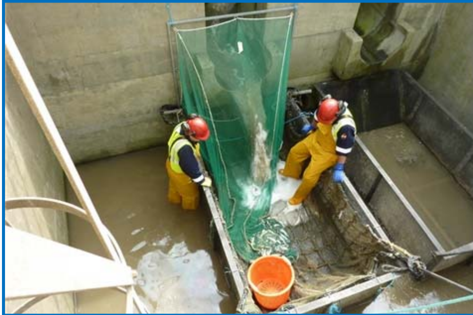
Figure 2.2 Placement of hourly sampling nets in the trash bin at Sizewell B, the position of the bulk net is shown.
